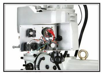
Figure 66. Control panel wiring.
